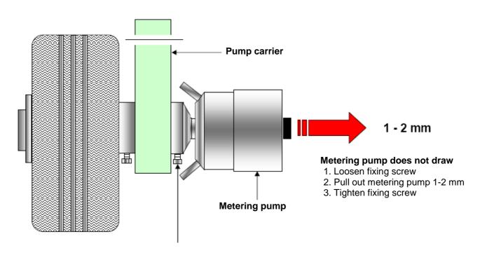
Clamping bush fixing screw
